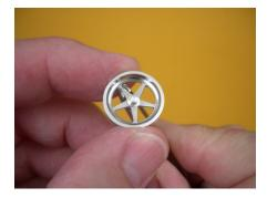
When satisfied that front and back inserts line up and are seated, use super glue around joint where insert and sleeve meet.
