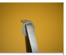
After making approximately 90-degree bend, fit bracket as tightly against outer circumference of rotor as possible.
