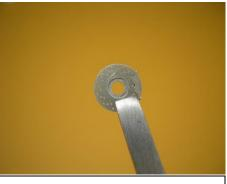
If bent properly, the hole in the middle of the bracket will be centered in hat locating hole in rotor.
