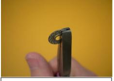
Finish bending of bracket by crimping over the rotor.
