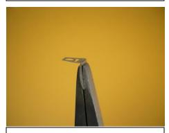
When bending, take care not to roll larger part of bracket over nose of pliers.
