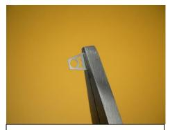
Use pliers that have square, smooth jaws that clamp evenly. Grip bracket at caliper end w/just a sliver of bracket visible next to the pliers.
