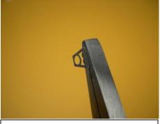
Holding bracket firmly with pliers, bend bracket while pulling slightly. You want the bend to take place as tight against the pliers as possible
