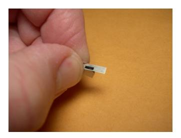
Locate and glue console cover to top of resin insert, making sure that outside edges are flush with outside edges of console body.
