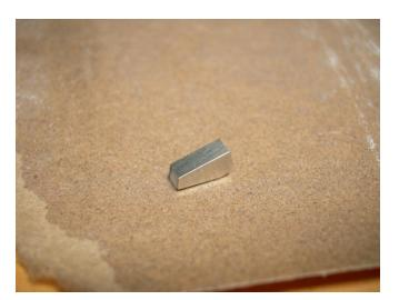
Surface top edge of resin insert so it is flush with top of console.
