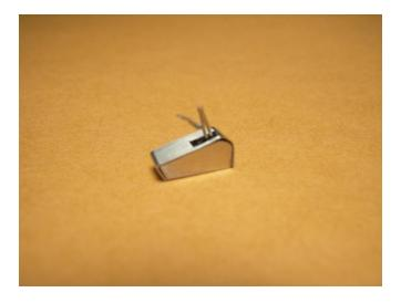
After wrapping edges of cover around front and rear ends and gluing to insert, trim or sand off any overlapping cover material. Install ball on top of lever.
